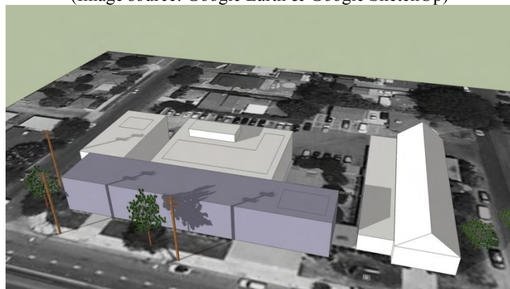
Figure 23: Shadow Analysis on a Large Non-Residential Parcel (Image source: Google Earth & Google SketchUp)
