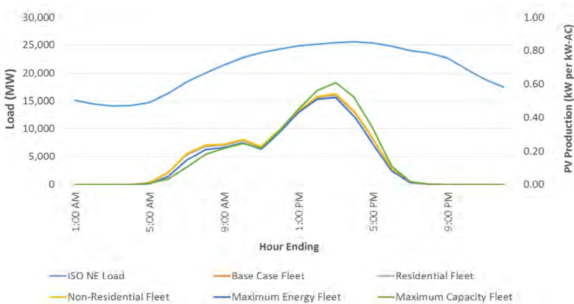
Figure 16. Normalized Fleet Production vs. ISO NE Load on 2012 Peak Load Day – July 17, 2012
